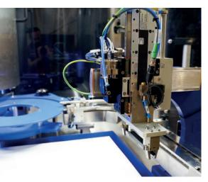
This modular solution allows the combination of distinct technologies within the same platform. The planar system is paired perfectly with indexing high-speed manipulators and continuous motion dials. Shuttles move according to the process time and quickly transport parts from one station to another without bottlenecks. Furthermore, the software constantly calculates the optimal path to direct the shuttles.
